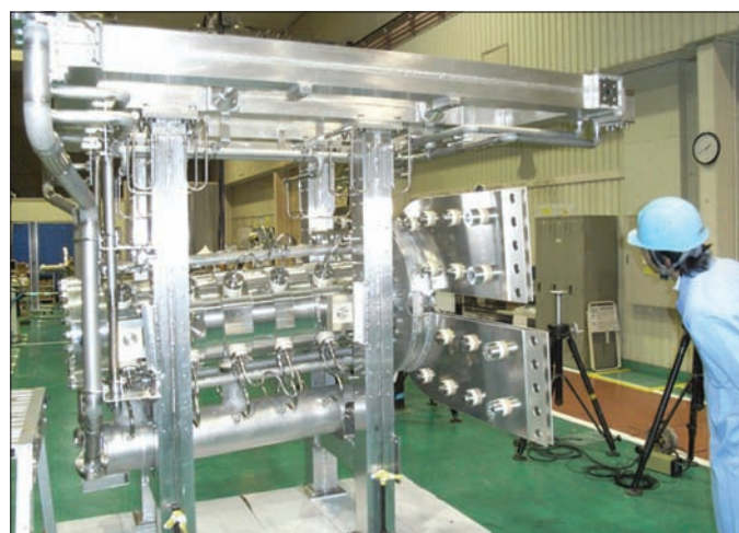
The first of three magnetic horns for T2K. This one will be combined with the target system at the start of the secondary beam line.
