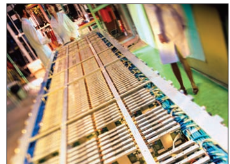
One of the supermodules for the ALICE TOF under assembly at CERN. (Courtesy A Saba for CERN.)
