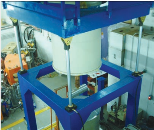
Fig. 4. The arrangement to test the thermoacoustic detection of particles on an ultracryogenic resonant antenna (left), which is sensitive enough to detect the impact of cosmic rays. The detector vibrates when it is hit by the full intensity of the Beam Test Facility beam (right). (Courtesy LNF-INFN.)
