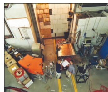
Fig. 2 (left). A BTF beam spot (on silicon microstrip detectors, 0.240 mm pitch). (Courtesy AGILE.) Fig. 3 (right). The BTF hall, showing the last dipole with the double beam exit. (Courtesy G Federici/LNF-INFN.)
