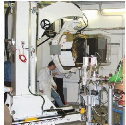
Fig. 5. The Italian Space Agency's AGILE payload during calibration runs with the BTF tagged photon beam. (Courtesy AGILE.)
