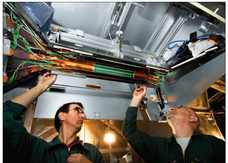
Top left: the detector element, a ladder, consists of a silicon-sensor matrix bump bonded to a ladder structure. Above left, middle right and above right: three views of the SPD barrel during assembly test.
